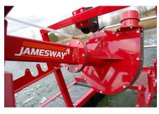
The large inlet on the 20" diameter impeller easily ingests debris.
