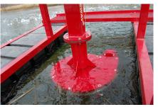
The lower bearing is never exposed to manure, resulting in long life and low maintenance.
