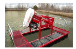
The lifting winch tilts the pump to make servicing quick and easy.
